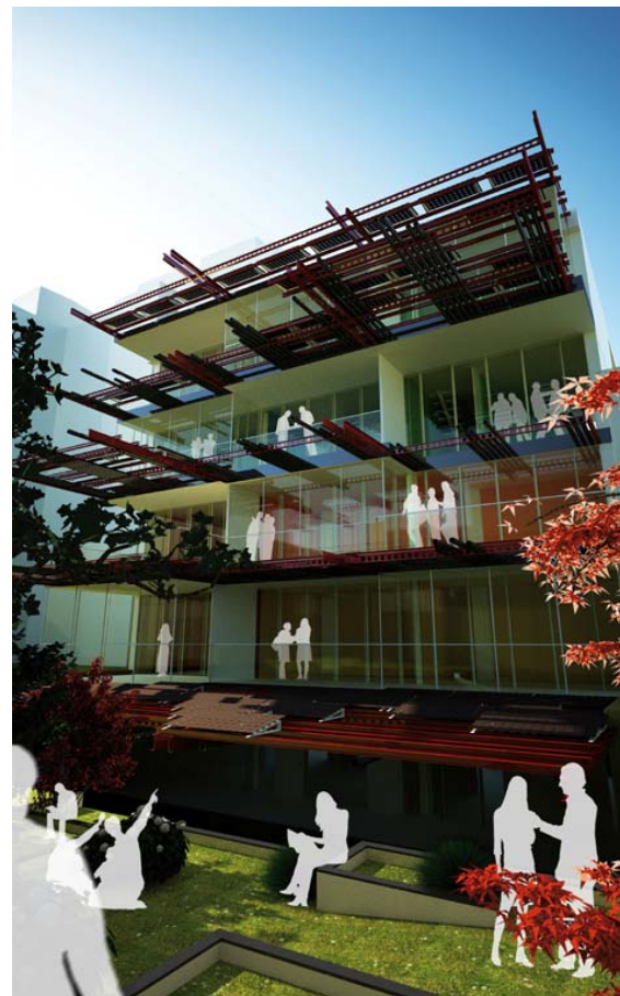
Figure 4: Degreen / case 1 / design: F. Lampis, M. Leo. E. Petriglia / the Southern facade with Photovoltaics
